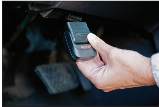
Figure 1: An on-board diagnostic device plugs into an OBD connector located within two feet of the steering wheel, under the dashboard.
